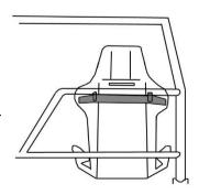
on 23cm square plate 3mm (min.) thick. This new section must not be constructed in a way that a drivers helmet can make contact with it. Material od and thickness as rest of roll cage.
