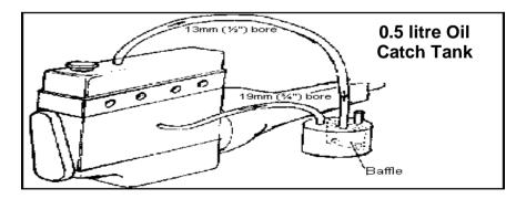
An oil catch tank, with a minimum capacity of 0.5 litres, must be fitted in the engine bay, and must have a minimum of two breather pipes connecting to it, one from the rocker box and one from the crank case. If the catch tank becomes ineffective during racing or practice, the car will be withdrawn from the event.
