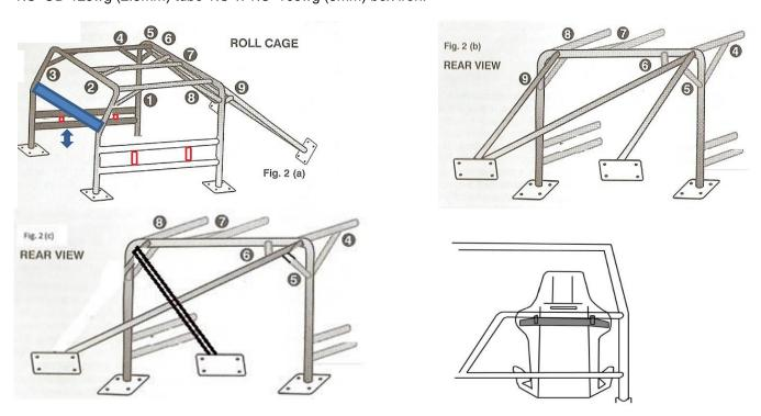
Corner gusset bars are included in the diagrams to be added as a means to add weight to the car if necessary.
