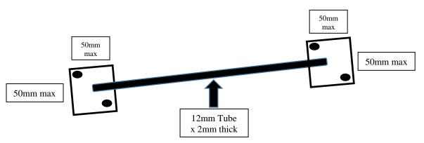
This is a bracket which you may put on a Corsa C from the chassis out to the front bumper to support the end of the bumper. This is the maximum size allowed and must be bolted and not welded in place with a maximum of 2 bolts each end.
