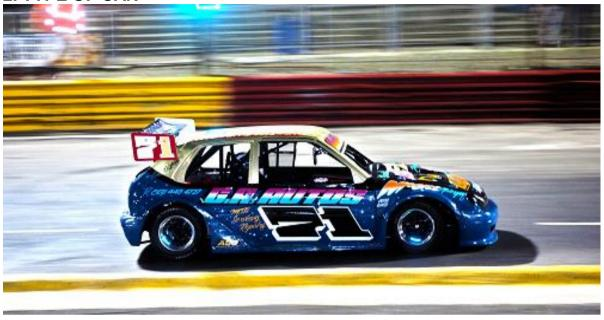
**A.** Any four-seater, front-engined, saloon or hatchback, constructed of steel, the overall length must not exceed 3988mm (157") and the overall width must not exceed 1702mm (67") when ready to race. Consideration will be given to any modern vehicle which falls outside these specified measurements in its original form, but can comply when prepared for racing, as follows:
